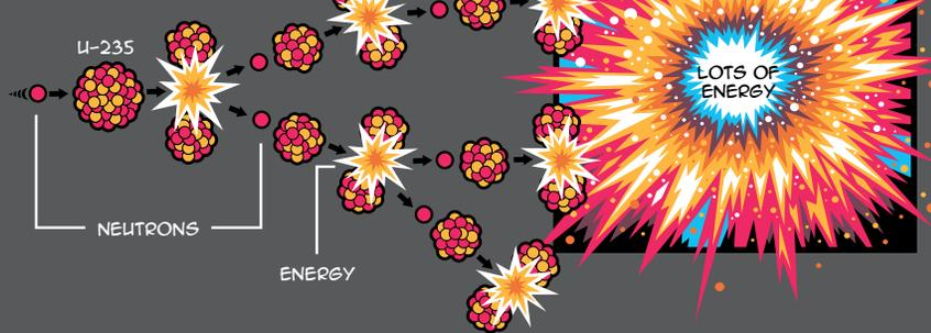
IS FIRED AT THE NUCLEUS OF THE ISOTOPE U-235. THIS EXTRA NEUTRON IN THE NUCLEUS MAKES THE ISOTOPE HEAVIER AND HIGHLY UNSTABLE. TO RELEASE THAT ENERGY, THE ISOTOPE SPLITS INTO TWO SMALLER ELEMENTS. IT ALSO RELEASES A FEW NEUTRONS IN THE PROCESS. THESE NEUTRONS GO ON TO COLLIDE INTO OTHER U-235 ISOTOPES, CAUSING A CHAIN REACTION (I.E., A NUCLEAR REACTION).
