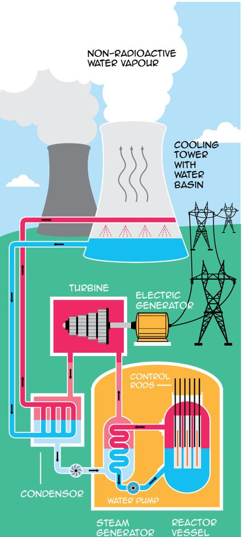
THIS HEAT BOILS WATER AND CREATES STEAM TO POWER THE GENERATORS THAT PRODUCE ELECTRICITY.
