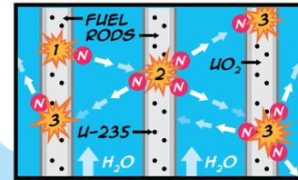
THE NEUTRONS RELEASED IN THE REACTION MOVE AT SPEEDS THAT MAKE IT DIFFICULT FOR THEM TO HIT OTHER ISOTOPES. TO MAKE SURE THE NUCLEAR REACTION CAN CONTINUE, THE NEUTRONS NEED TO BE SLOWED DOWN, OR "MODERATED." WATER IS USED AS A MODERATOR.
